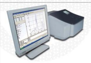
Using the UVProbe software provided makes it possible to control the UV-1800 with a PC. UVProbe is an all-in-one software product that includes the following four functions: Spectrum mode, Photometric (quantitation) mode, Kinetics (time-course) mode, and a superb Report Generator.
