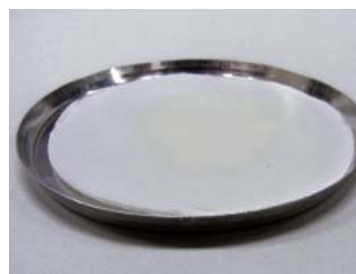
(After measurement) The moisture has evaporated from the milk, and the remaining fats have yellowed slightly.
