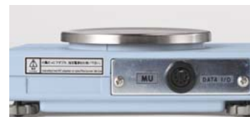
Data transfer port of ELB Series
