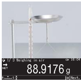
First measure the empty weight.
