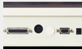
Data transfer port of BW-K/BX-K Series
