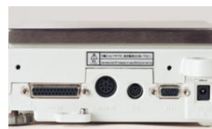
Data transfer port of UW/UX Series
