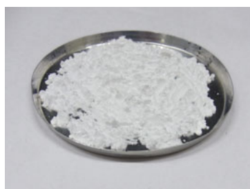
(Before measurement) The sample powder was spread evenly over the pan.
