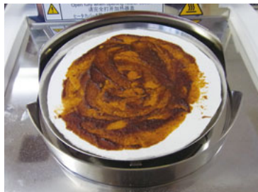
Fiberglass sheet coated with dengakumiso and loaded in the MOC63u
