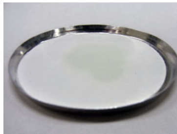
(Before measurement) 1 g of milk was dripped on to a fiberglass sheet for liquid measurements.
