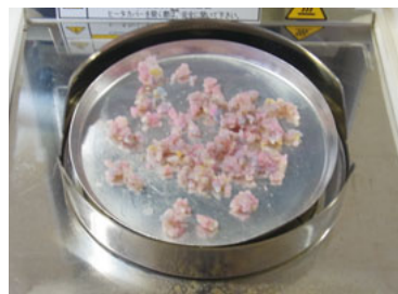
Ground up boiled fish paste loaded in the MOC63u
