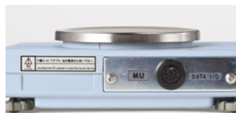
Data transfer port of ELB Series
