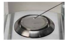
When the measurement spoon is electrically charged, and bringing it near the pan affects the numerical value
