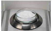
When the powder in the Petri dish is electrically charged, and the numerical value fluctuates
