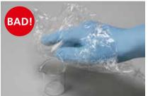
Plastic wrap adheres to rubber gloves, making it difficult to work with.
